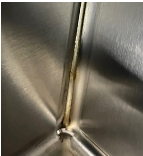
Fillet Weld with Filler Material
